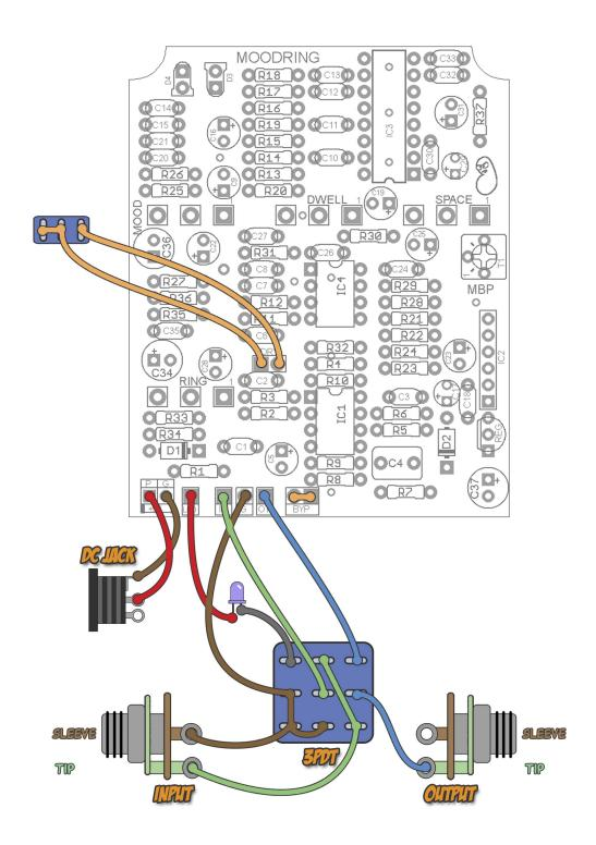
Be sure to jumper the two "BYP" pads as shown and omit R8.
