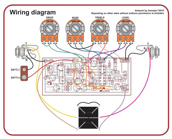
Orange jumper wires only for single sided board!
