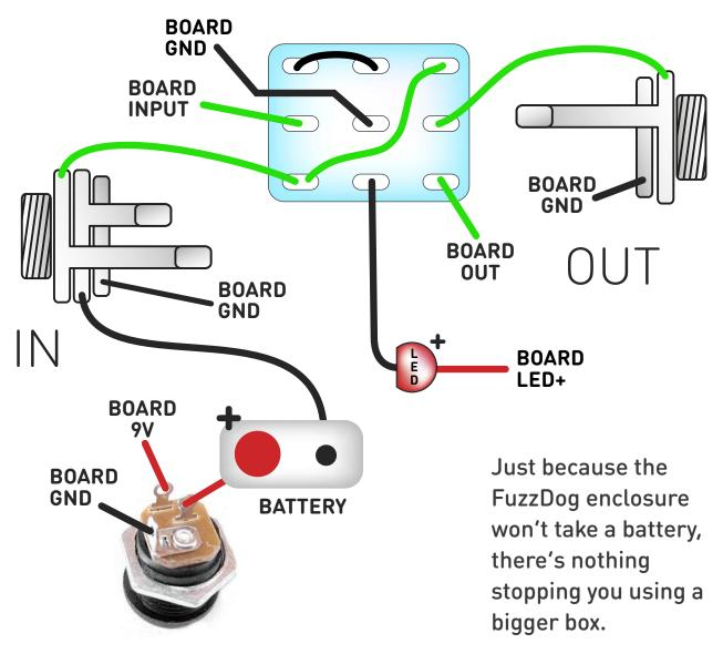
This circuit is standard, Negative GND. Your power supply should be Tip Negative / Sleeve Positive. That's the same as your standard pedals (Boss etc), and you can safely daisy-chain your supply to this pedal.
